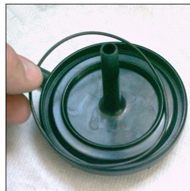
Fig. 3 - Place o-ring into the filter housing
