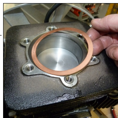
Fig. 1 - Lower valve gasket
