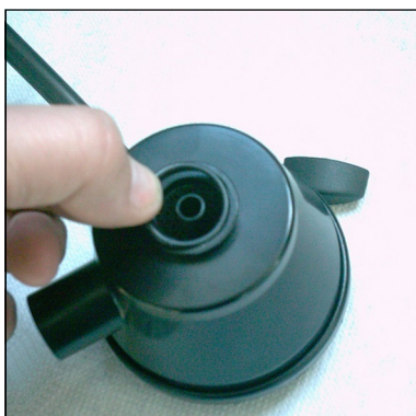
Fig. 4 - Place o-ring into the groove
