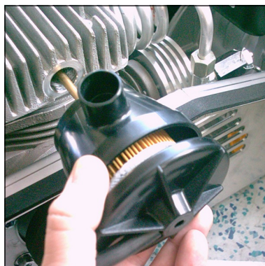
Fig. 2 - Pull out filter housing carefully
