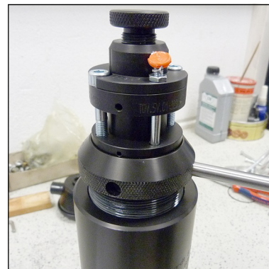
Fig. 1 - Remove/screw in filter cover
