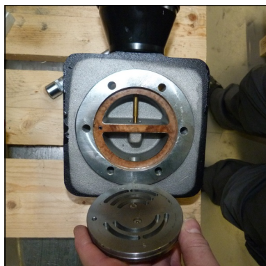
Fig. 2 - Correct position of inand outlet valve
