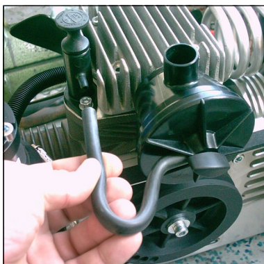
Fig. 1 - Pull off ventilation hose at the oil fill port
