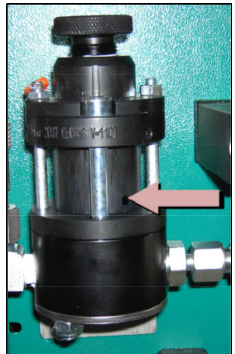
Figure 1: Position for oil refill
