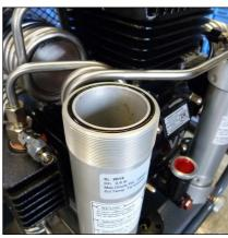
Fig. 2 - Filter housing without filter cover
