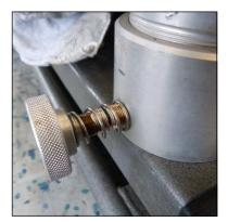
Abb. 6 - O-ring, condensate drain valve
