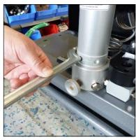
Abb. 3 - Turn off filter housing
