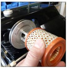
Fig. 3 - Change intake filter
