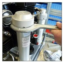
Fig. 1 - Filter housing with filter tool
