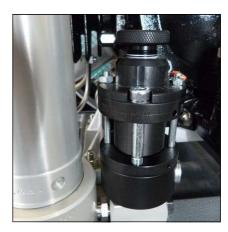
Fig. 2 - Safety valve 3rd stage
