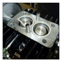
Fig. 4 - Change valve gasket
