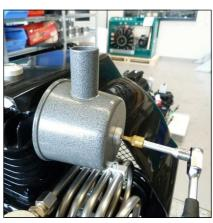
Fig. 1 - Iloosen mounting screw
