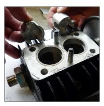
Fig. 3 - Valve bracket positioning
