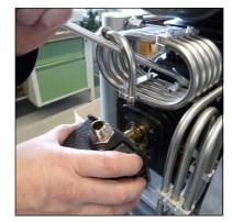
Fig. 3 - Remove valve head
