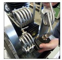
Fig. 4 - Remove valve head with inlet and outlet valve
