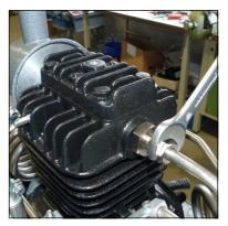
Fig. 7 - Tighten pipe connections
