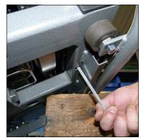
Fig. 3 - Loosen both bottom mounting screws
