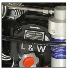
Rotation direction arrow on the compressor block
