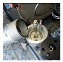
Abb. 4 - Remove lock ring
