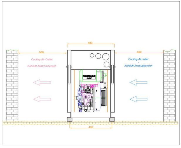
Fig. Ventilation via ventilation stack
