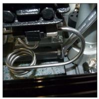
Fig. 2 - Loosen pipe connections of the filter housing
