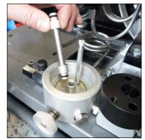
Abb. 5 - Remove duct collar and change o-rings
