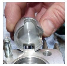
Fig. 1 - Outlet valve holder 1st. stage
