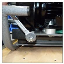
Fig. 3 - Turn clamp nut until correct Vbelt tension
