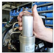
Fig. 3 - Filter cartridge and spring
