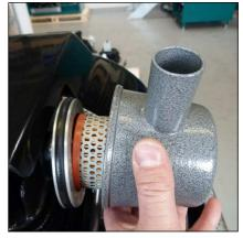
Fig. 2 - Remove intake filter housing cover
