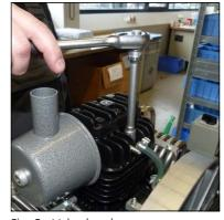
Fig. 3– Valve head screws
