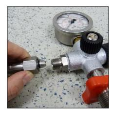
Fig. 2 - O-ring at the filling hose
