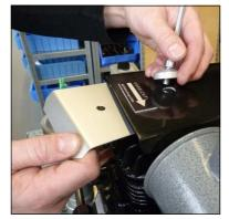
Fig. 2 - Remove protection plate
