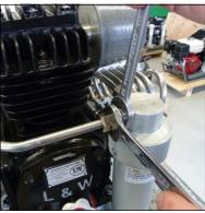
Fig. 1 - Loosen pipe connections of the water separator
