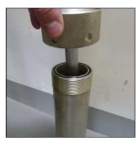
Abb. 4 - Remove lock ring and change o-ring
