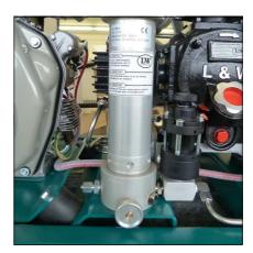
Fig. 2 - Oil- / water separator 3rd stage
