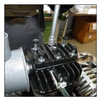
Fig. 4 - Valve head cover screws
