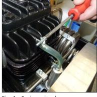
Fig. 1 - Spring wire clamp
