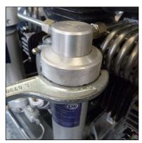
Abb. 5 - Tighten lock ring
