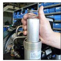
Abb. 2 - Remove filter cartridge
