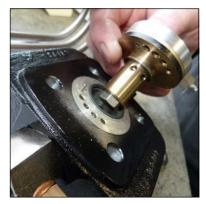
Fig. 4 - Ensure correct valve position (centre pin)
