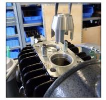
Fig. 6 - Inlet valve braket
