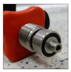
Fig. 1 - O-ring at the filling valve
