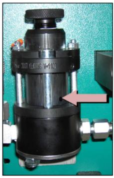
Figure 1: Position for oil refill
