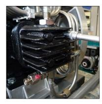
Fig. 2 - Loosen valve head screws
