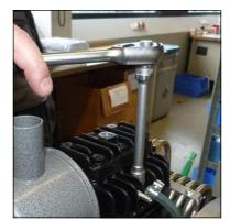
Fig. 6 - Tighten valve head
