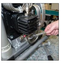
Fig. 1 - Loosen pipe connections
