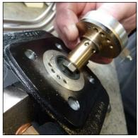
Fig. 5 - Ensure correct valve position (centre pin)
