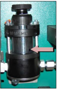
Figure 1: Position for oil refill
