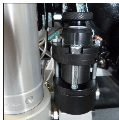
Fig. 2 - Safety valve 3rd stage
