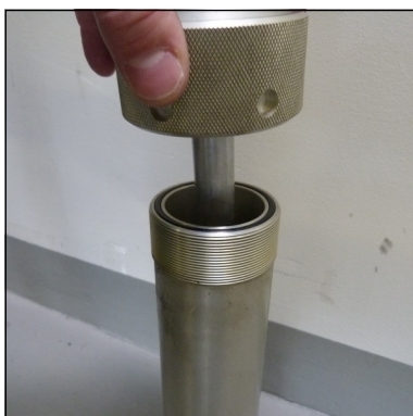
Fig. 4 - Remove lock ring and change o-ring
