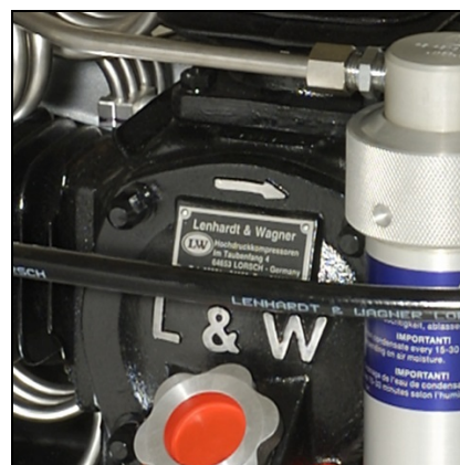
Rotation direction arrow on the compressor block
