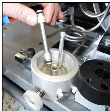
Fig. 5 - Remove duct collar and change o-rings
