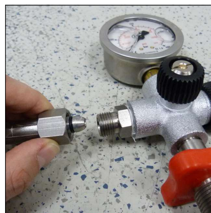
Fig. 2 - O-ring at the filling hose
