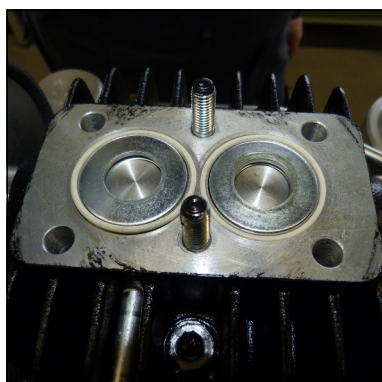
Fig. 5 - Spring plate inside the valve head
