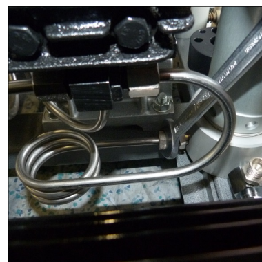
Fig. 2 - Loosen pipe connections of the filter housing
