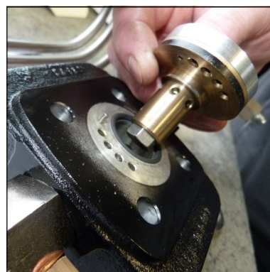
Fig. 5 - Ensure correct valve position (centre pin)
