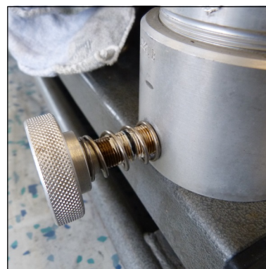
Fig. 6 - O-ring, condensate drain valve
