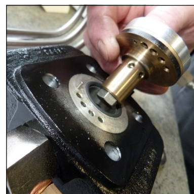
Fig. 4 - Ensure correct valve position (centre pin)
