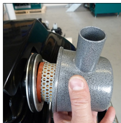
Fig. 2 - Remove intake filter housing cover
