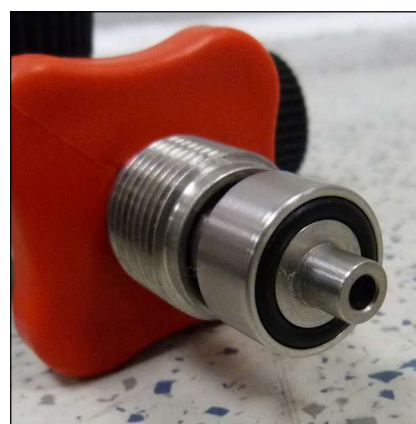
Fig. 1 - O-ring at the filling valve
