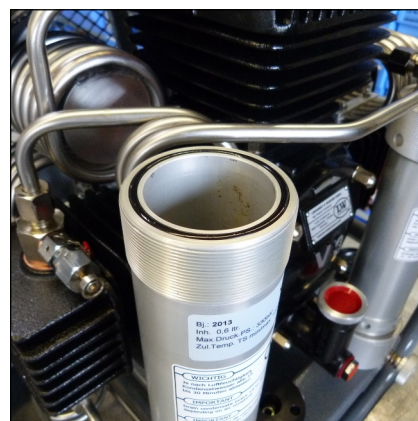
Fig. 2 - Filter housing without filter cover
