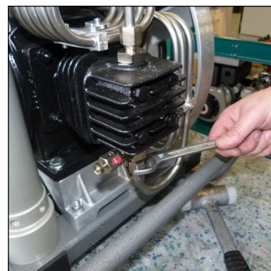
Fig. 1 - Loosen pipe connections
