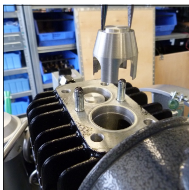
Fig. 6 - Inlet valve bracket
