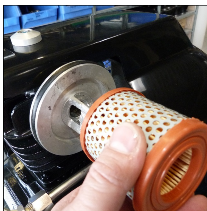
Fig. 3 - Change intake filter
