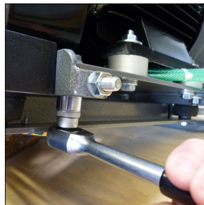
Fig. 1 - Loosen mounting screws of the motor flange
