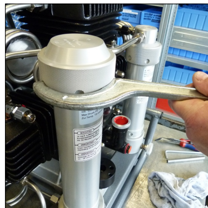
Fig. 1 - Filter housing with filter tool
