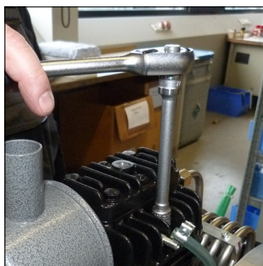
Fig. 6 - Tighten valve head
