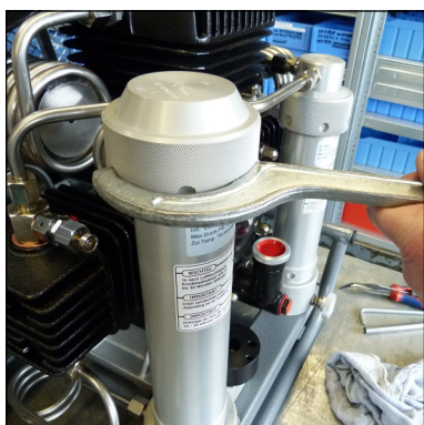
Fig. 1 - Open filter cover
