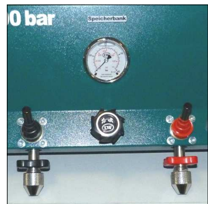
Fig. 1 - Hand wheel valve and pressure gauge
